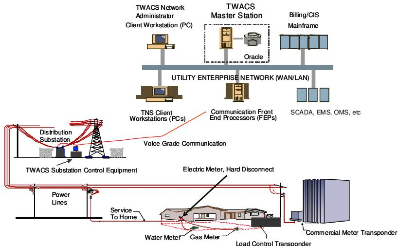
Outbound signalling is communication from the substation to the end-point devices and inbound signalling for end-point device communication detected at the substation. This is a low bandwidth technology that relies on clever use of concurrency techniques to deliver its service. This is a proprietary technology.
