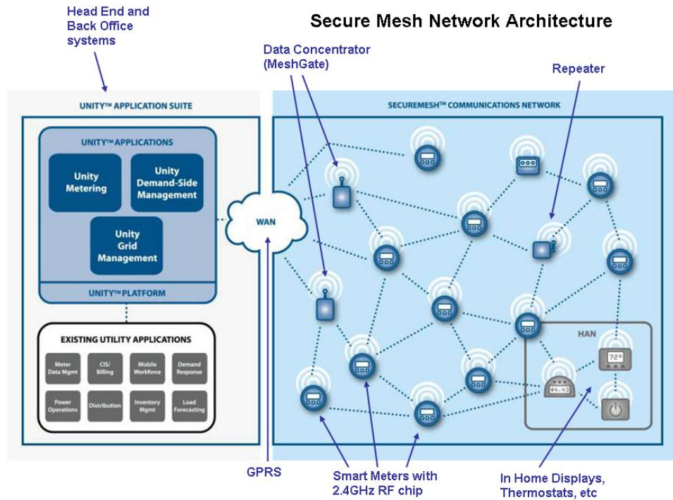
The key components are the meter including the comms module, the repeaters, the MeshGate (Collector/Data Concentrator), the WAN modem and SerViewCom (the head end). These components and their functions are described in more detail below.
